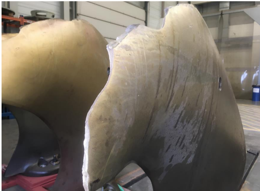
Image 4.1 Mechanical damage of the blade. Author's photograph.
